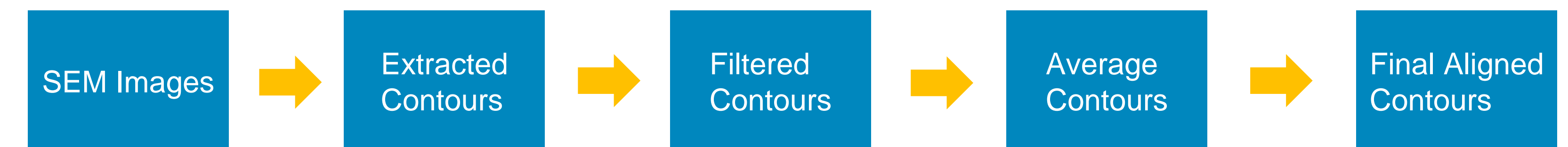
Figure 6: Schematic flow of contour extraction and post-processing
