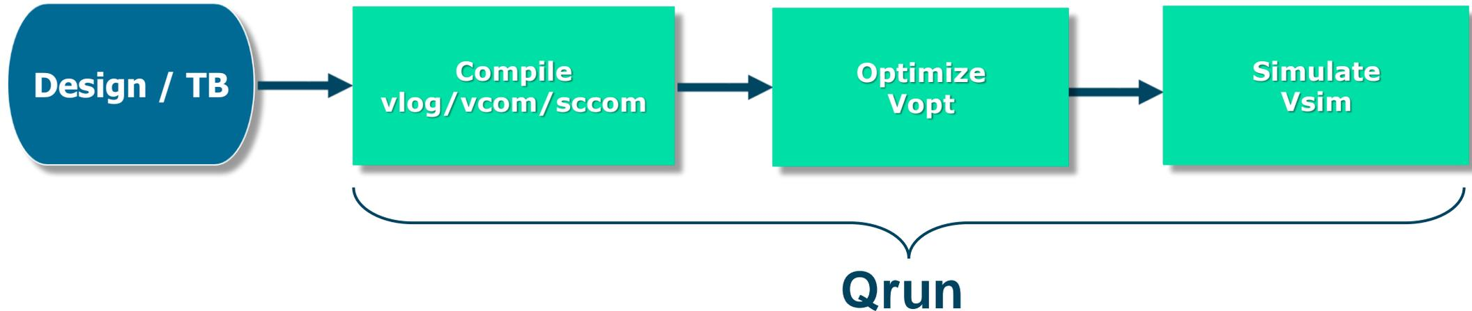
The Qrun utility simplifies the use of Questa tools to compile, optimize and simulate a design by taking all input files and options, and then automatically executing the correct tool and command-line arguments for each file.
