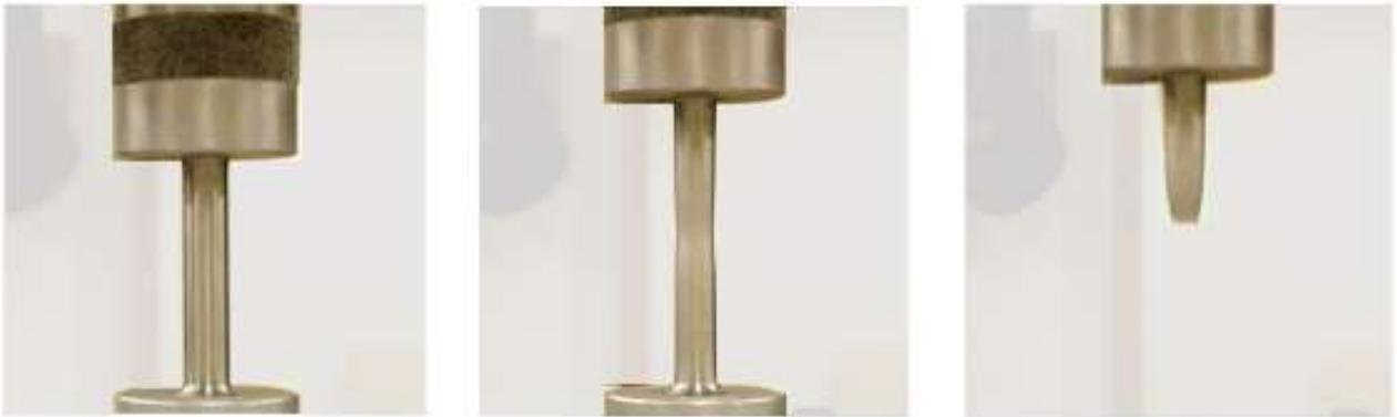
Picture 1: Stress/strain test of metal coupon sample. Left: Original sample. Middle: Sample with necking. Right: Sample with failure
