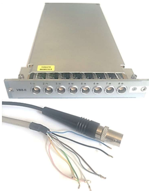
Picture 1: VB8-II card and with Open Wire (other end is LEMO) cable and BNC wire (other end is LEMO) cable
