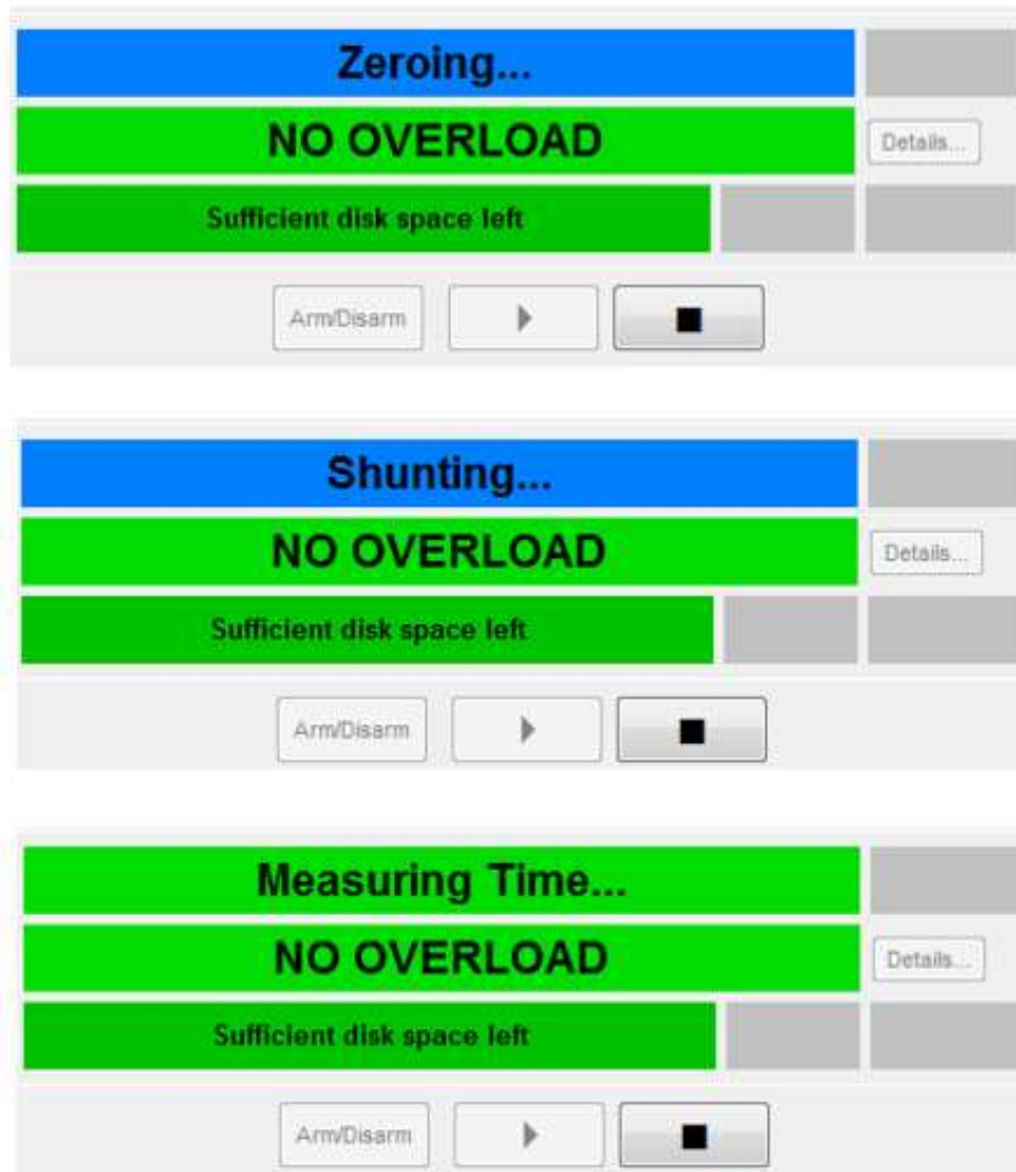
Picture 16: Shunt measurement sequence automatically takes zero and shunt measurements (default 3 seconds each) before and after acquisition. Status is indicated by blue message.
