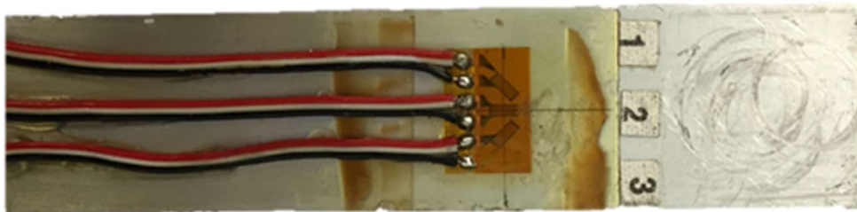
Figure 5: Rosette Strain Gauge consists of three co-located strain gauges.
