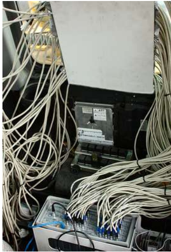
Figure 1: The long cables of a strain measurement system with low level voltage signals are susceptible to electrical interference from nearby power sources.
