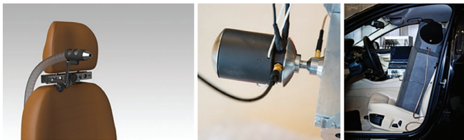
Figure 13: (From left to right): LMS Qsources mid- and high-frequency volume velocity source, integral shaker and low-frequency volume velocity source.
