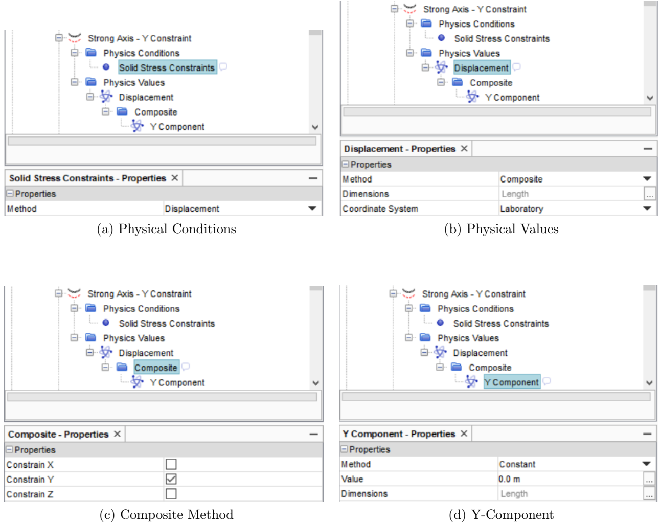
Figure 7: Curve Segment Definition Example: Strong Axis
