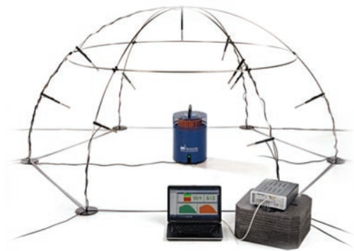
Figure 1: Reference sound source measured with the use of a half-hemisphere microphone array.
