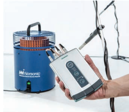
Figure 6: The reference sound source is being measured with the use of a hemisphere and mobile acquisition system.
